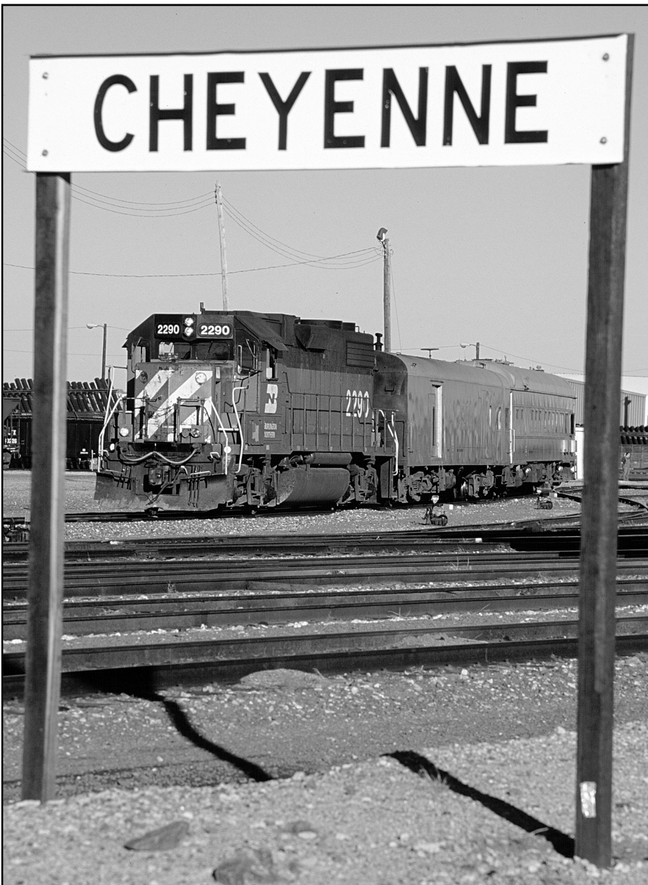
BNSF tested the Front Range Subdivision trackage on June 6, 2002. BNSF GP38-2 2290 handled track geometry cars BNSF 86 & 85. The train left Cheyenne, WY, about 8:00 AM via Fort Collins to Denver, CO. – Photo © Chip.
